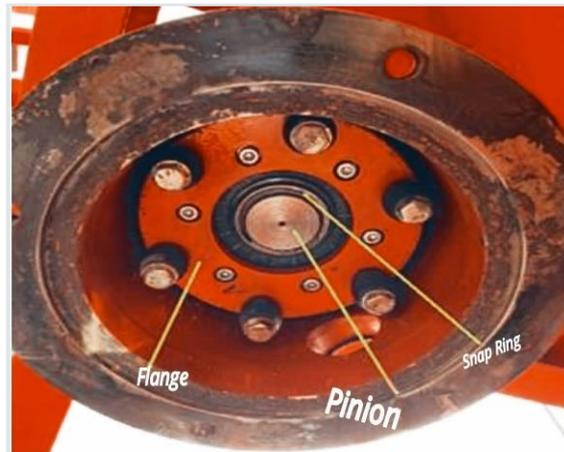
Gambar 7. Freewheel clutch
